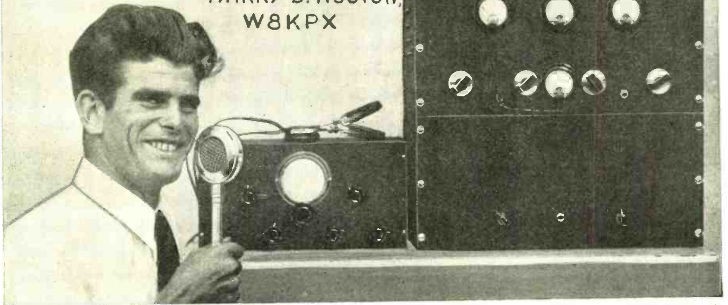
This picture shows the 35-watt transmitter at the top of the rack, while just below it appears the modulator. Cabinet seen at left of picture is the station receiver.
